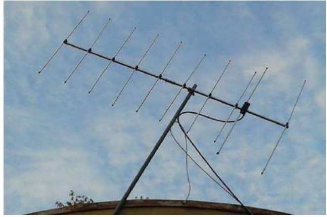
Figure 3 – Vertically polarized Yagi antenna.
