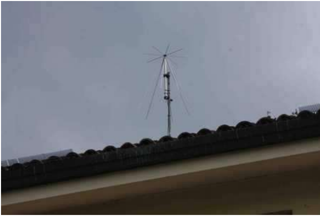
Figure 14 – “Discone” antenna.
