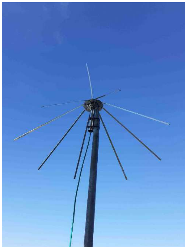
Figure 17 – Testing of the self-built ground plane antenna.
