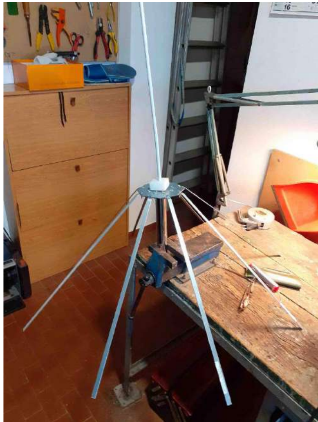
Figure 15 – Self-built ground plane antenna “Carmelina_143”.
